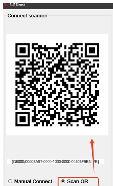
2.2.3 After the scanner powered on, scan the QR code shown on the app (There is no need to switch the scanner into Bluetooth BLE mode, the connection will be done under any mode after scanning this code.). After scanning the code, the connection will be automatically done. It will be shown successfully connect on the app.
