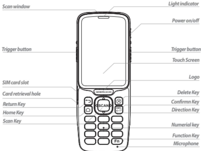
**Fn** key can switch numbers, uppercase letters, lowercase letters and function keys. You can reference detailed status according to changes on the up right corner.
