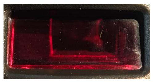
Step5. Check cleaning result of the window slice - no scratches on the surface of window slice, and the scanner can work normally, then this time cleaning is effective.
